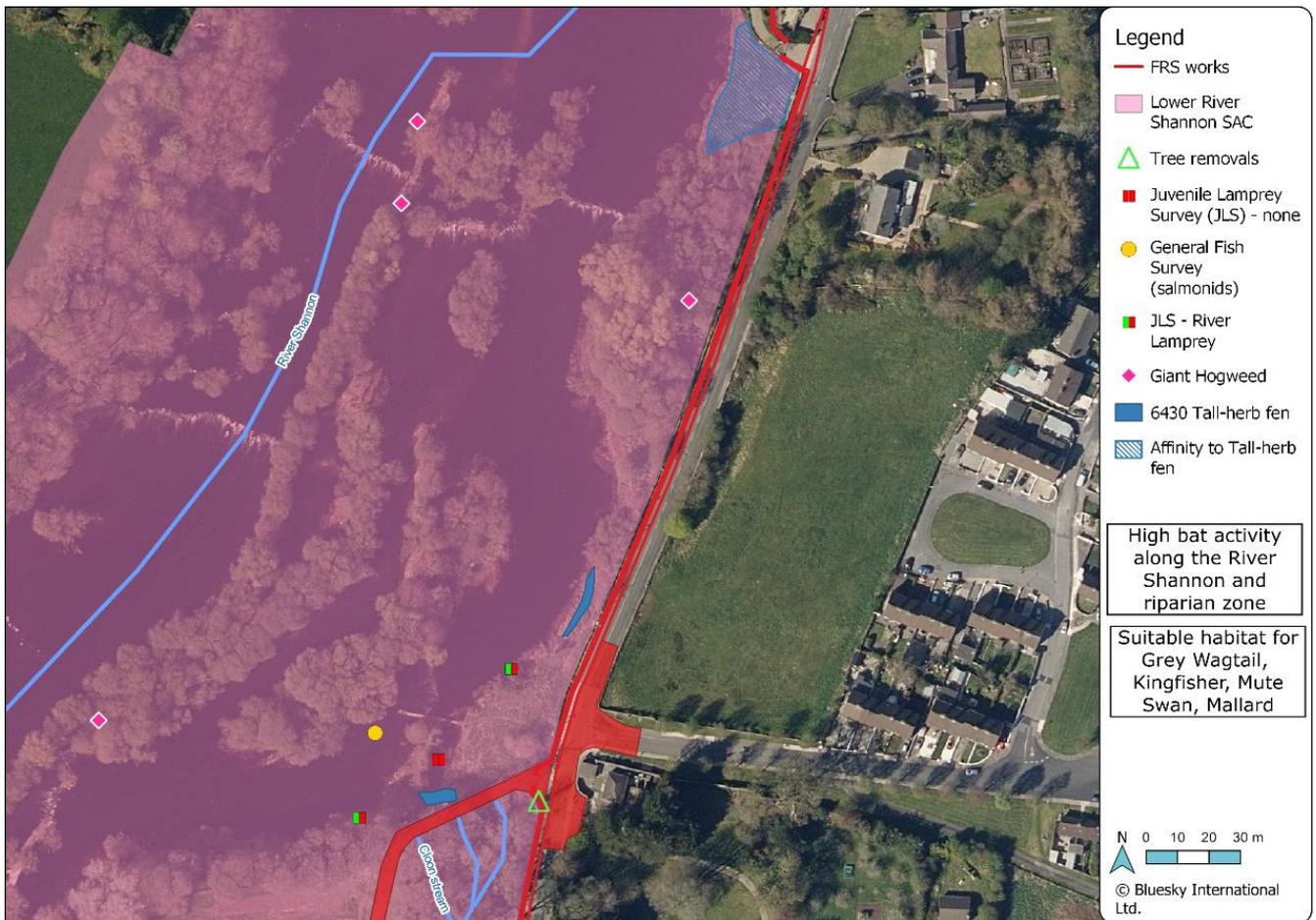
**Figure 8-37: Overview of FRS construction works and screened-in ecological features at Mall Road (phase 1)**
