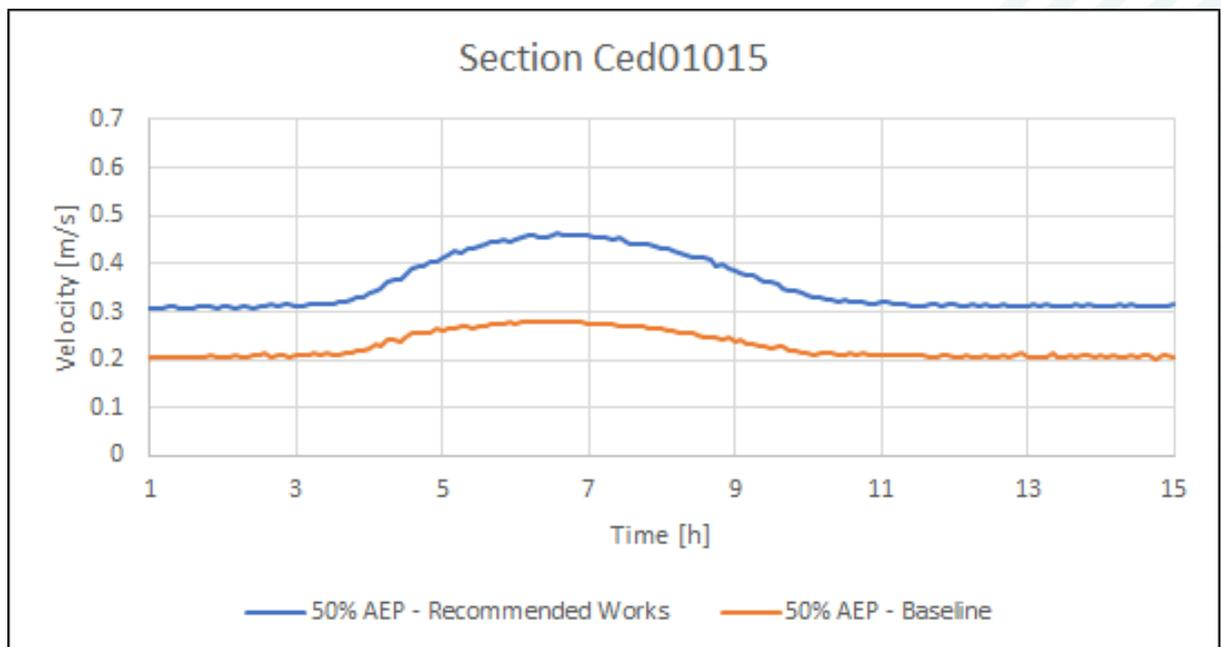
**Figure D0-31: 50% AEP Velocities – Section Ced01015 (Downstream of railway line)**
