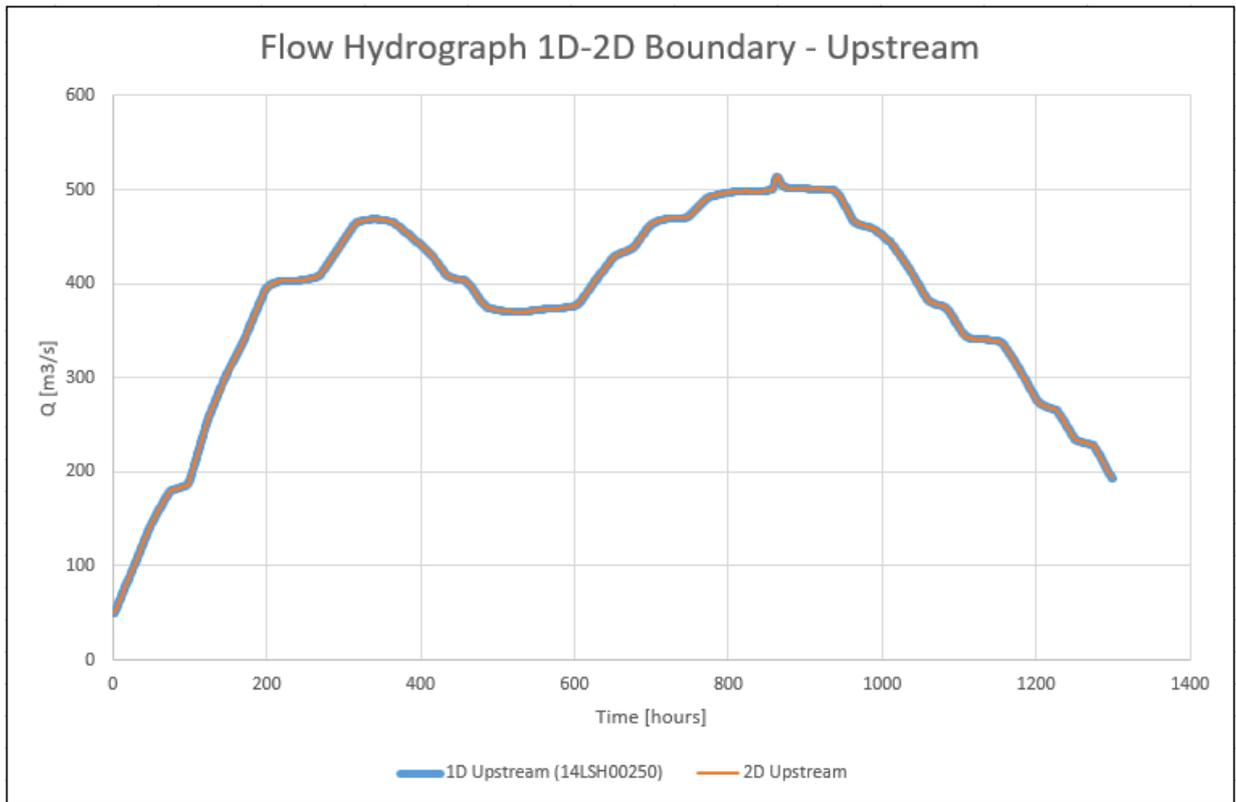
**Figure 2-11: Flow Hydrographs Modelled at the Upstream 1D-2D Boundary (1% AEP with 345 m<sup>3</sup>/s headrace flow - “504 event”)**
