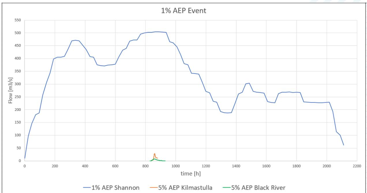
**Figure 2-5: Old Shannon downstream of Parteen Weir 1% AEP (after headrace flow of 345 m<sup>3</sup>/s to Ardnacrusha – “504 event”)**
