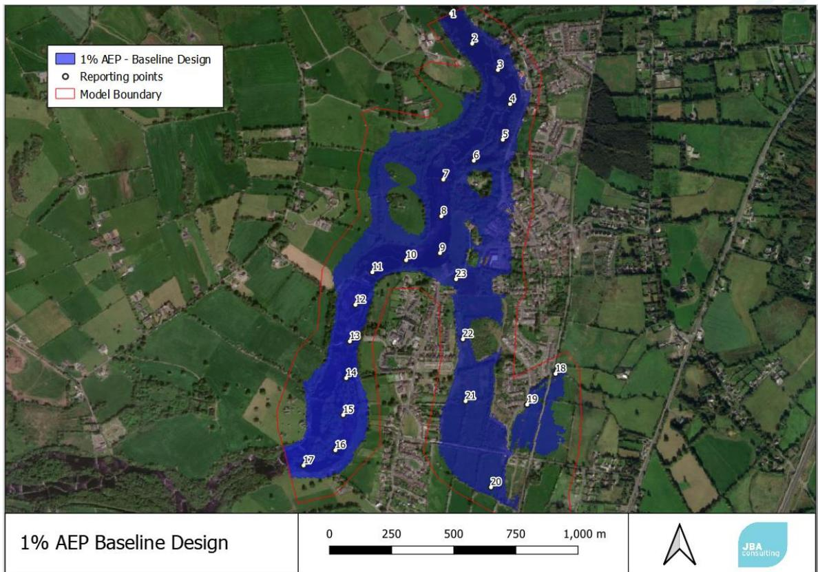
**Figure 5-2: 1% AEP Baseline design event (258 m<sup>3</sup>/s headrace flow)**
