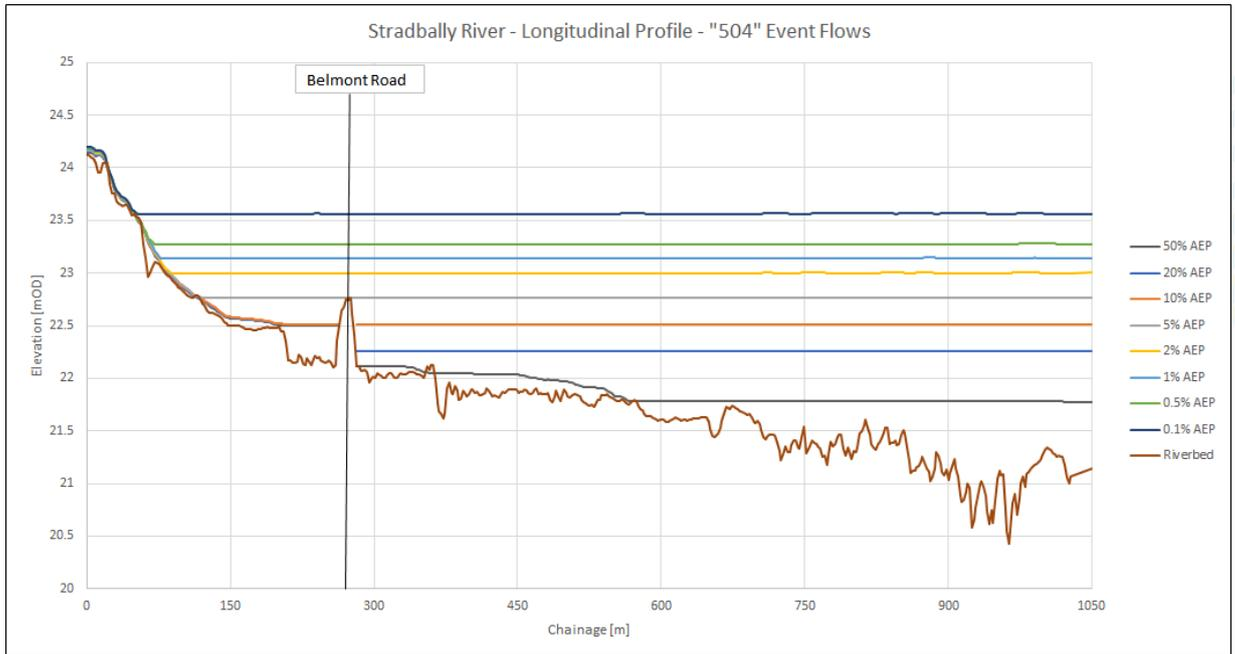
**Figure B-13: Stradbally Stream – Longitudinal Profile “504” event (354 m<sup>3</sup>/s headrace flow)**
