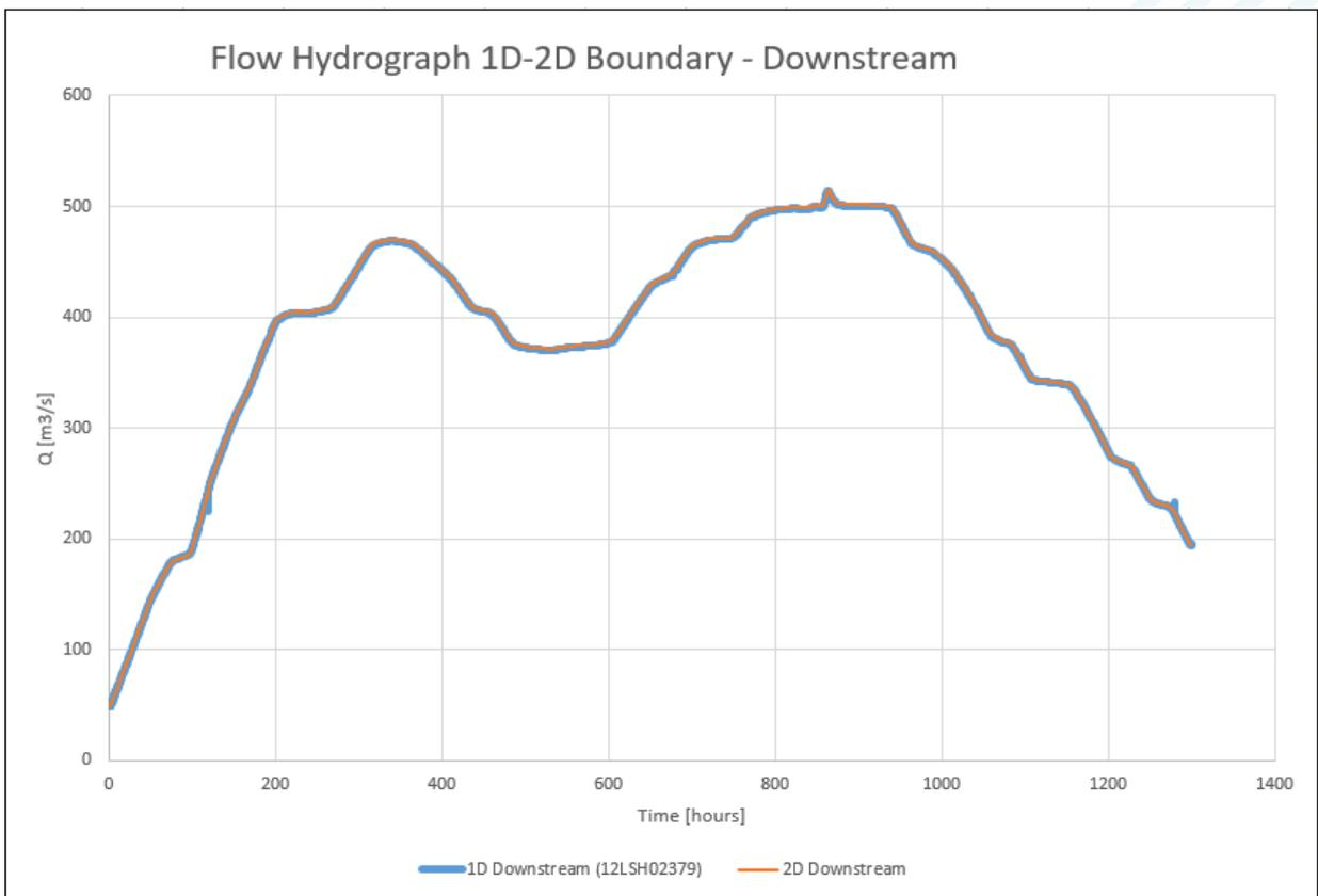
**Figure 2-12: Flow Hydrographs Modelled at the Downstream 1D-2D Boundary (1% AEP with 345 m<sup>3</sup>/s diversion - “504 event”)**
