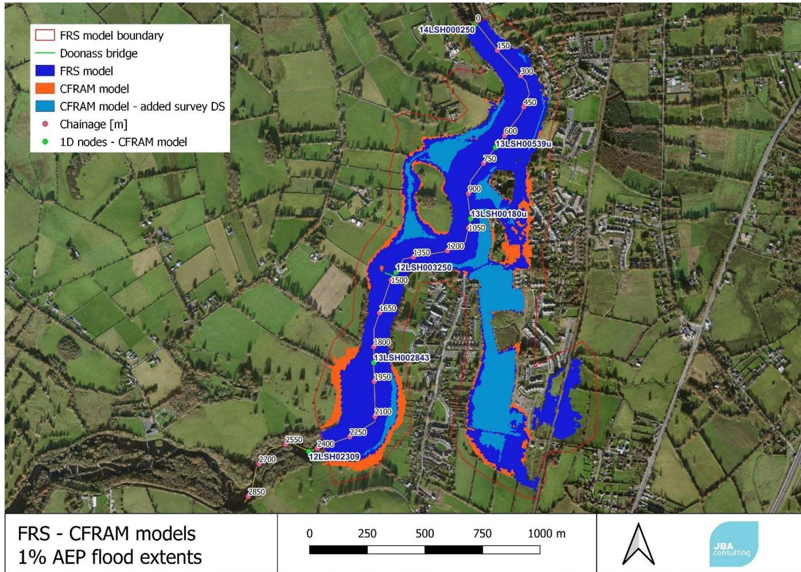
**Figure 3-7: 1% AEP Flood extents – FRS and CFRAM models**
