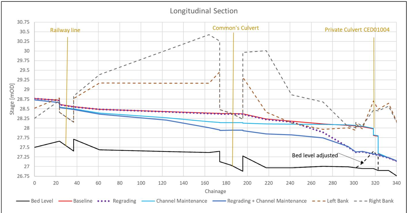
**Figure D0-28 –Longitudinal Section - 1% AEP Peak Water Levels**
