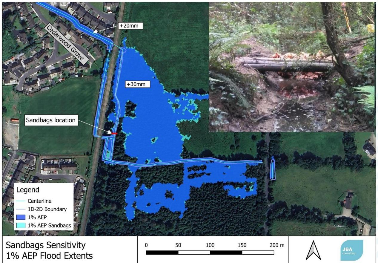
**Figure D0-17: Sandbags Sensitivity Test**
