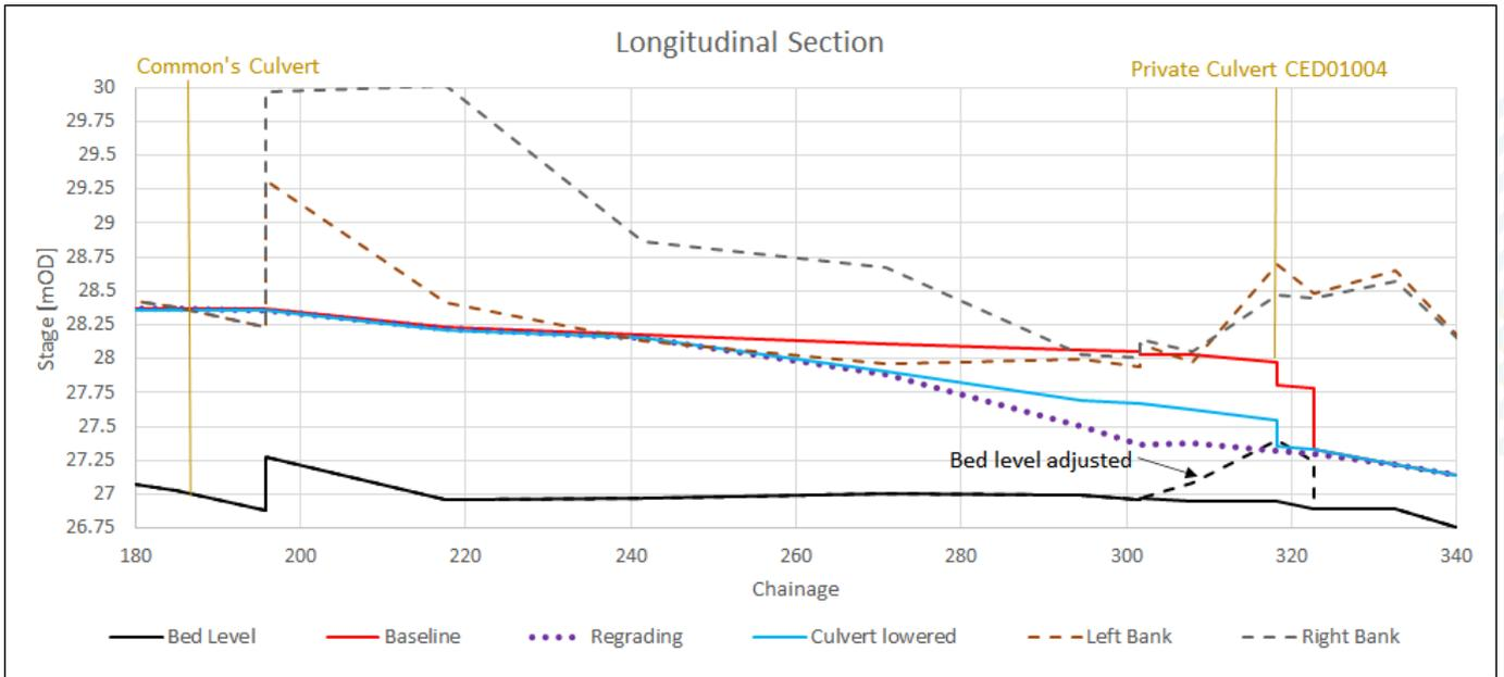
**Figure D0-26: Longitudinal Section – Culvert Testing**
