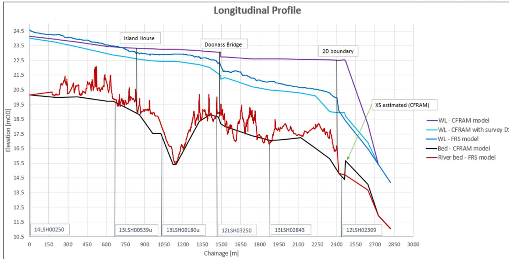
**Figure 3-8: 1% AEP (with 345 m<sup>3</sup>/s headrace flow to Ardnacrusha) Longitudinal profile– FRS and CFRAM water levels**
