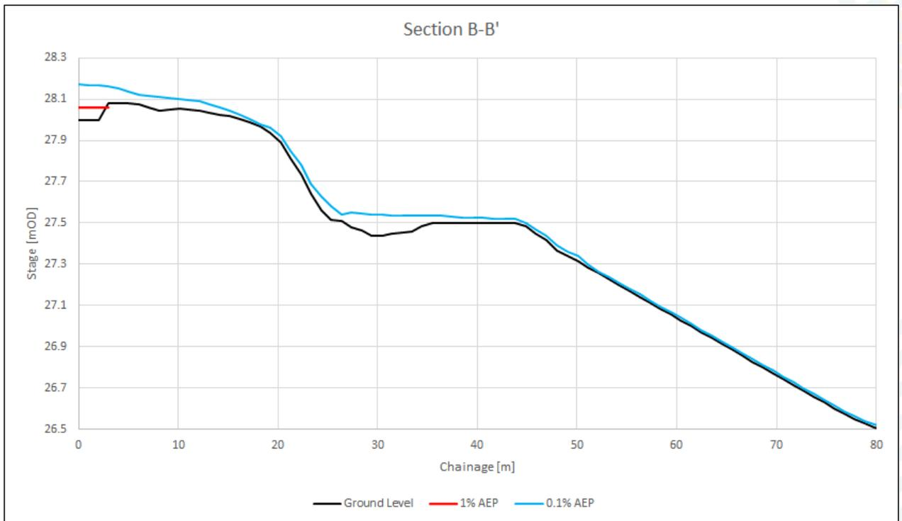
**Figure D0-8: Section B-B' – 1% and 0.1% AEP levels**
