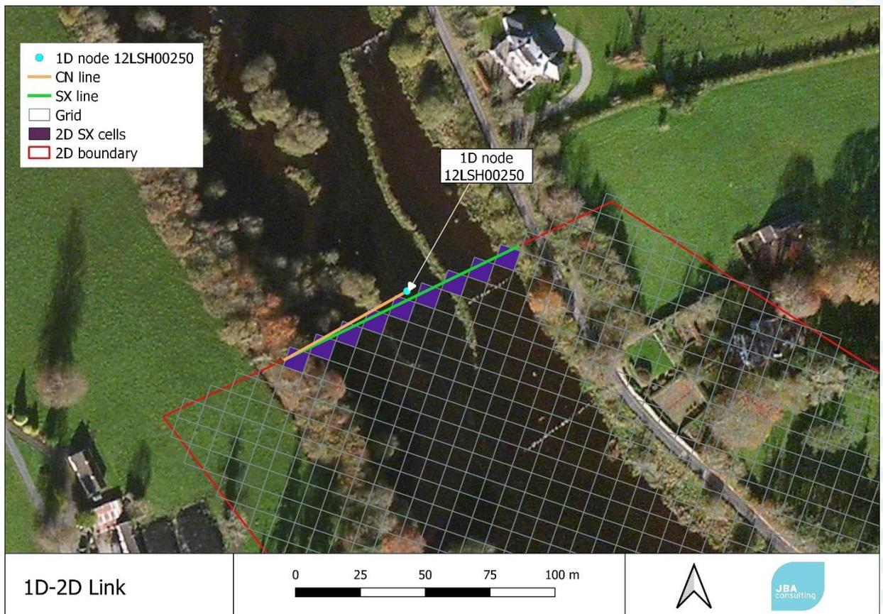
**Figure 2-10: Linking between 1D and 2D models**
