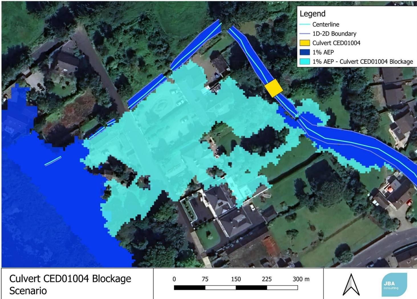
**Figure D0-15: 1% AEP – Culvert CED01004 Blockage Scenario**
