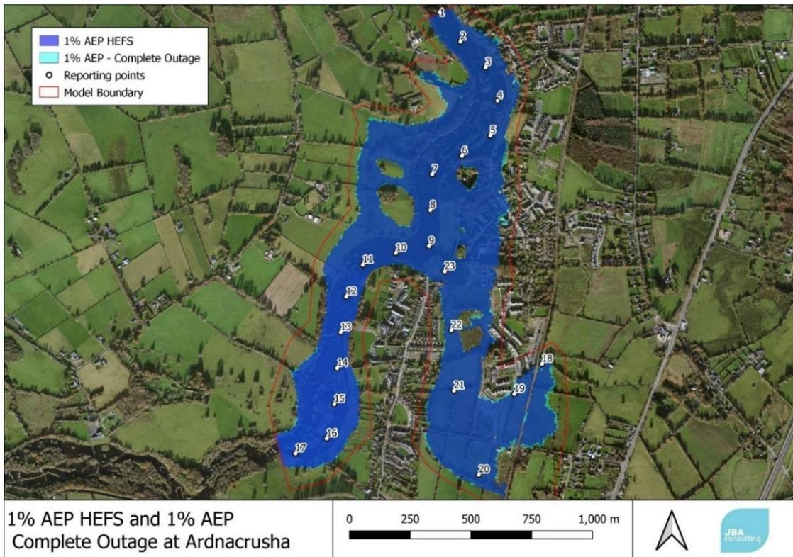
**Figure B-15: 1% AEP HEFS for “504” event (standard operational conditions - 345 m<sup>3</sup>/s headrace flow) and 1% Complete Outage at Ardnacrusha (zero headrace flow)**
