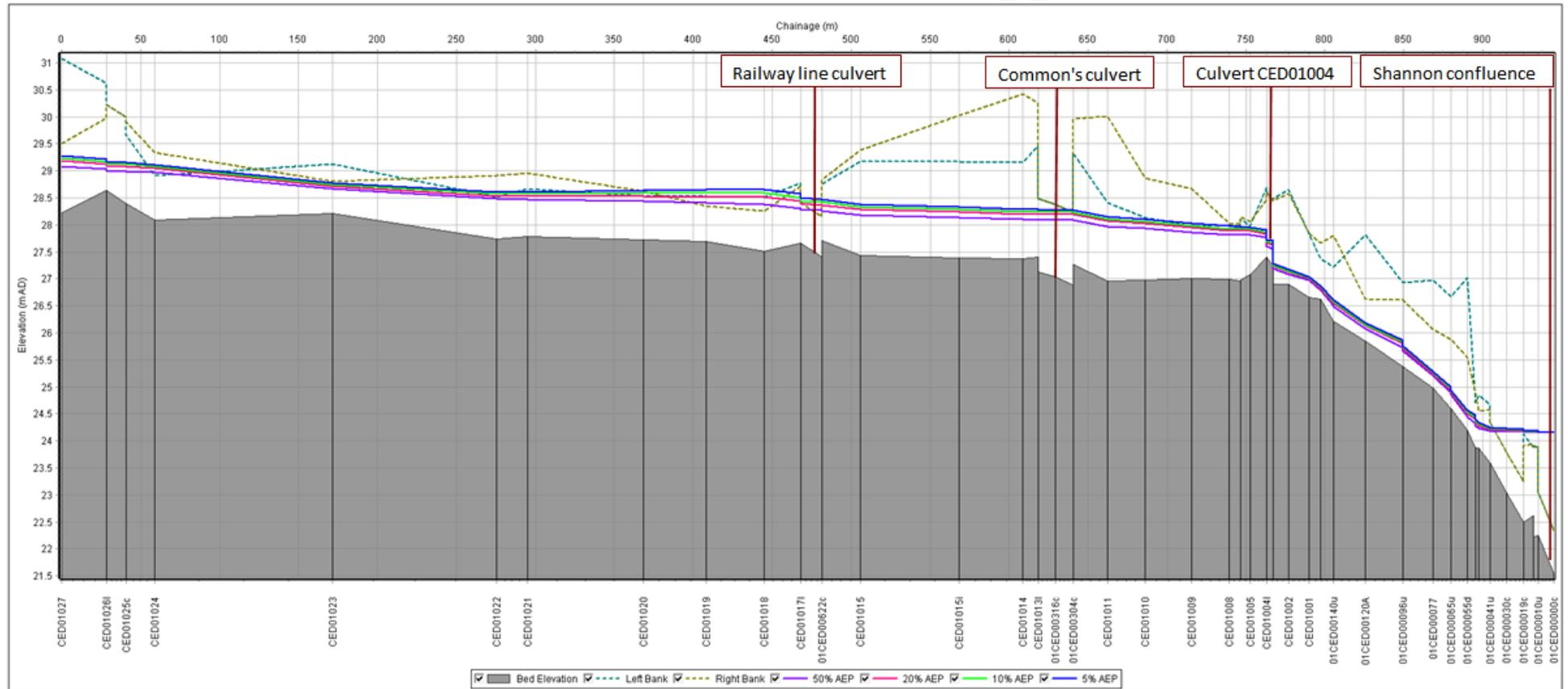
**Figure D0-23: Water Levels 5%, 10%, 20% and 50% AEP Events – Longitudinal Section**
