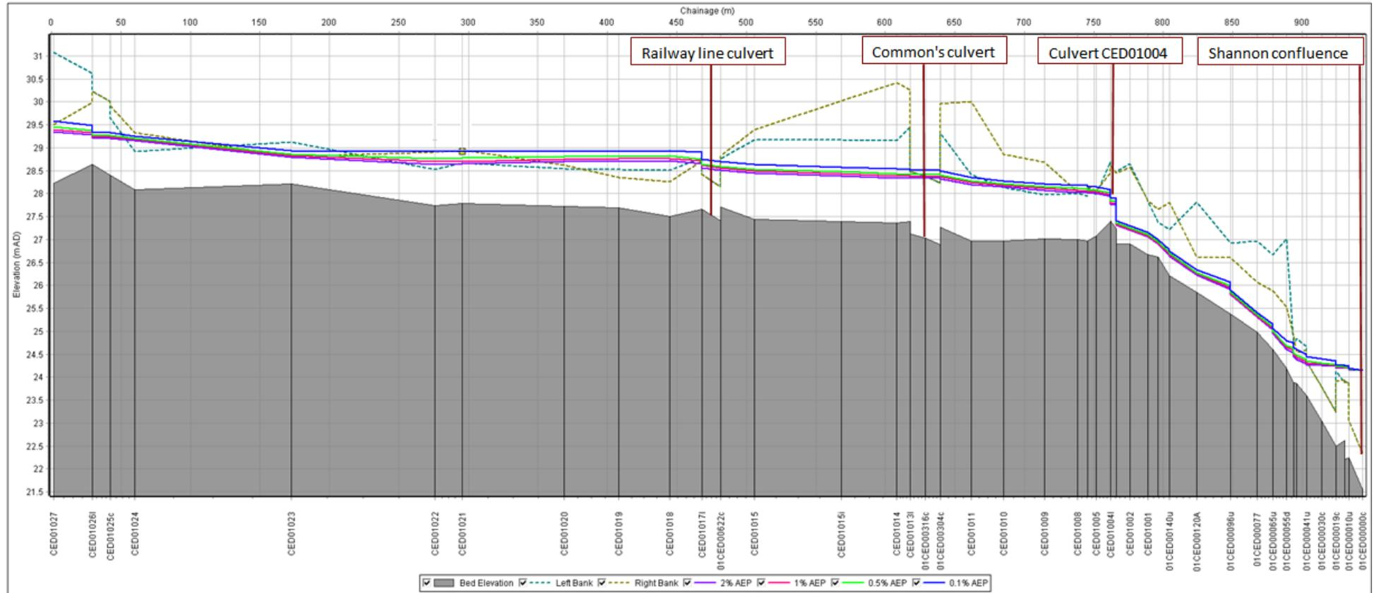
**Figure D0-24: Water Levels 0.1%, 0.5%, 1% and 2% AEP Events – Longitudinal Section**
