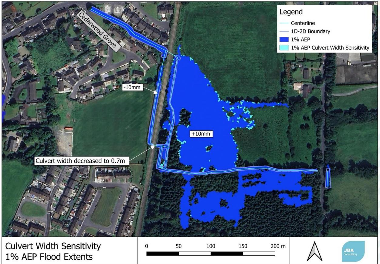
**Figure D0-20: Southern Culvert Width Sensitivity**
