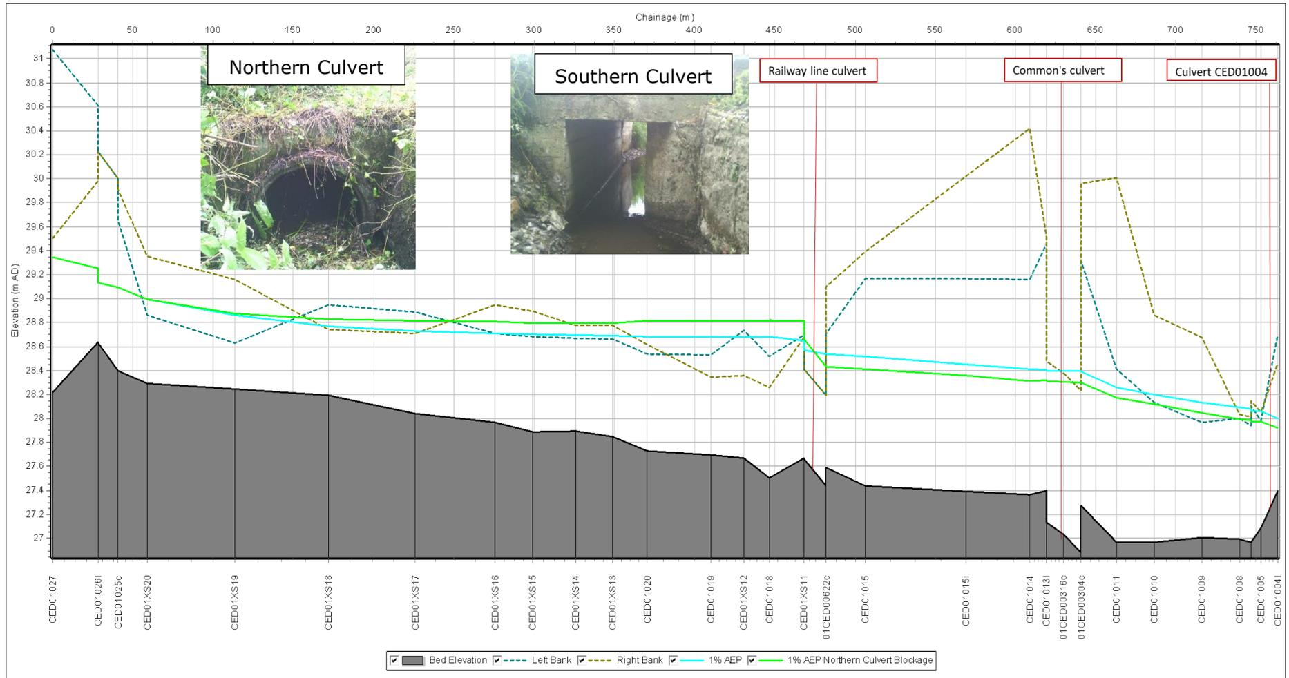
**Figure D0-12: 1% AEP Longitudinal Section - Railway line culvert blockage**
