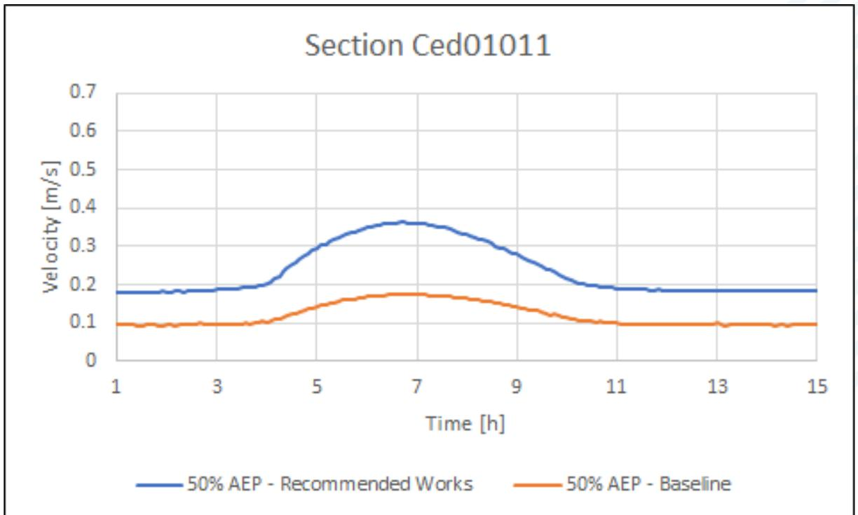
**Figure D0-33: 50% AEP Velocities – Section Ced01011 (Downstream of Common’s Road)**
