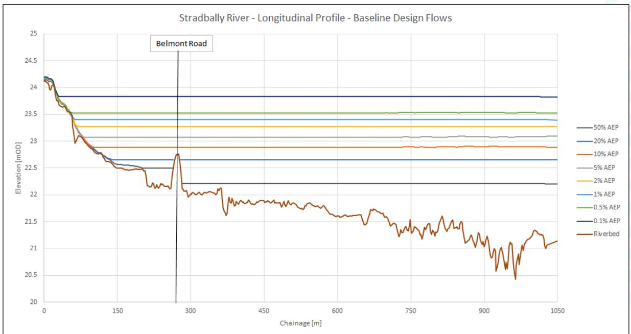
**Figure B-14: Stradbally Stream – Longitudinal Profile – Baseline Design Event (258 m<sup>3</sup>/s headrace flow)**
