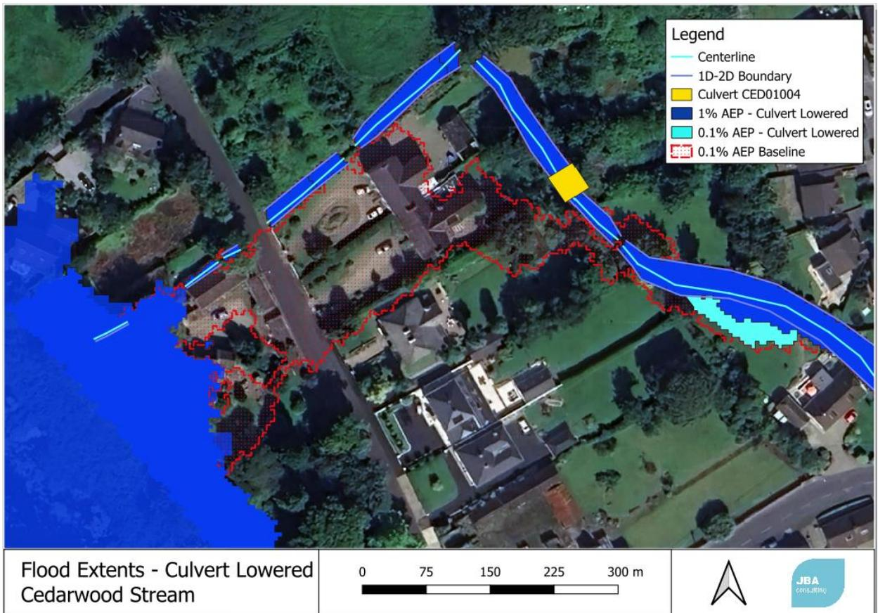
**Figure D0-25: 1% and 0.1% AEP Flood Extents – “Culvert Lowered” Scenario**
