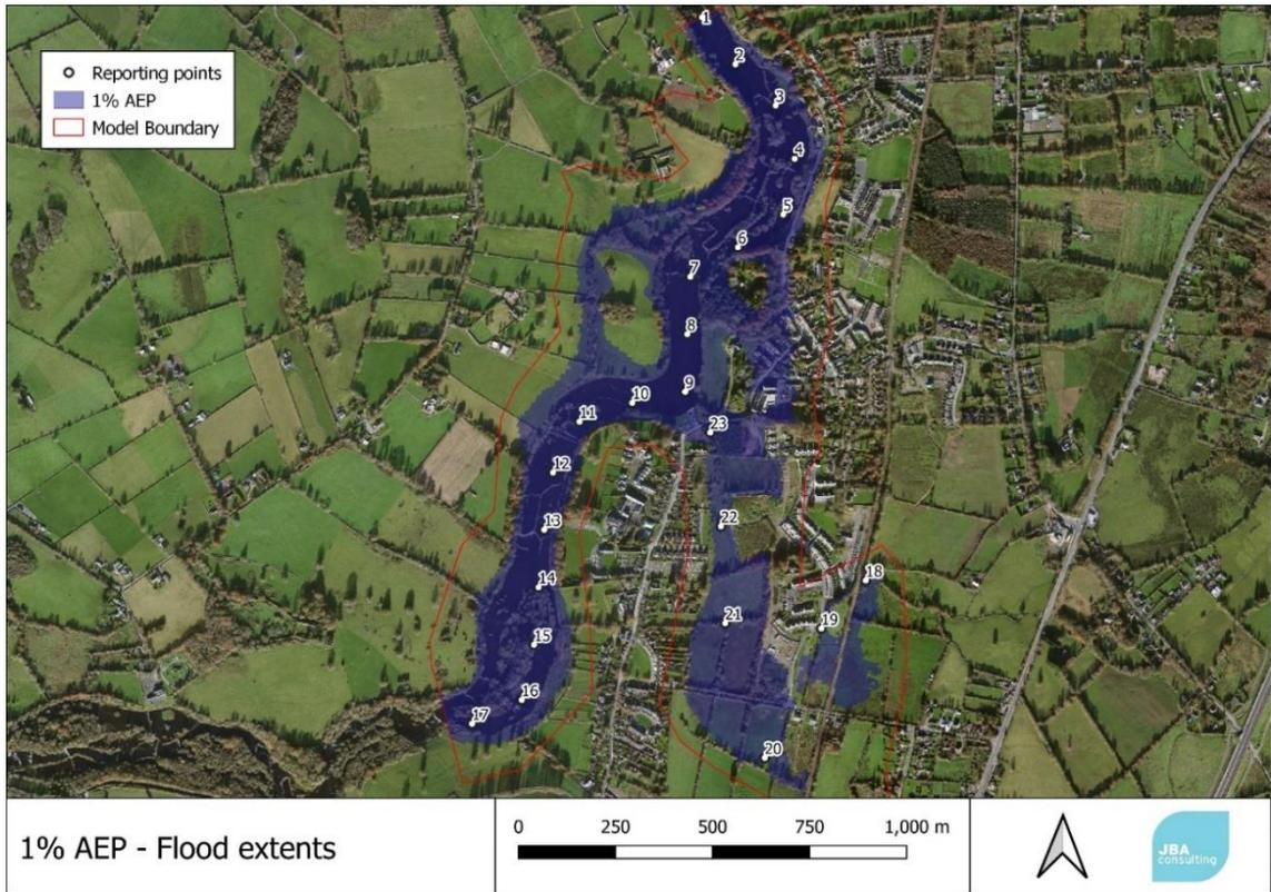
**Figure 5-1: 1% AEP for "504" event (345 m<sup>3</sup>/s headrace flow)**
